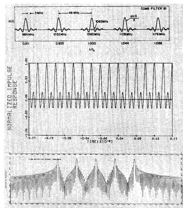
**Figure 6a. (top)** Frequency response to be realized.
